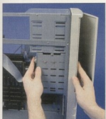
Any computer is pretty useless without a floppy drive. So, it's time to put the floppy disk into the tower case's drive cage and slot it into position
