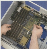
With the A1200 motherboard in position and securely screwed down, the Zorro slot busboard is plugged into the motherboard via the adapter
