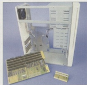
Apart from some boring nuts, bolts and screws, the Tower A1200 consists of these three main components which will turn your A1200 into a real power beast.
